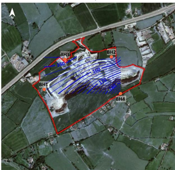
Figure 6.15: Groundwater Contours 2021 (aerial imagery from 2020). Groundwater elevations given in mAO.
