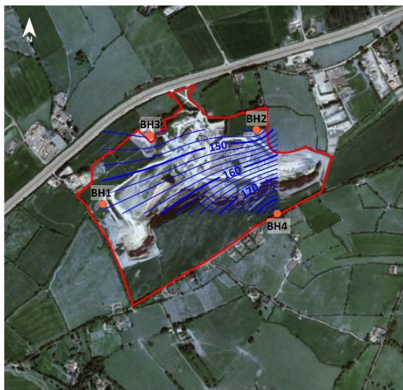
Figure 6.14: Groundwater Contours 2020 (aerial imagery from 2020). Groundwater elevations given in mAOD.
