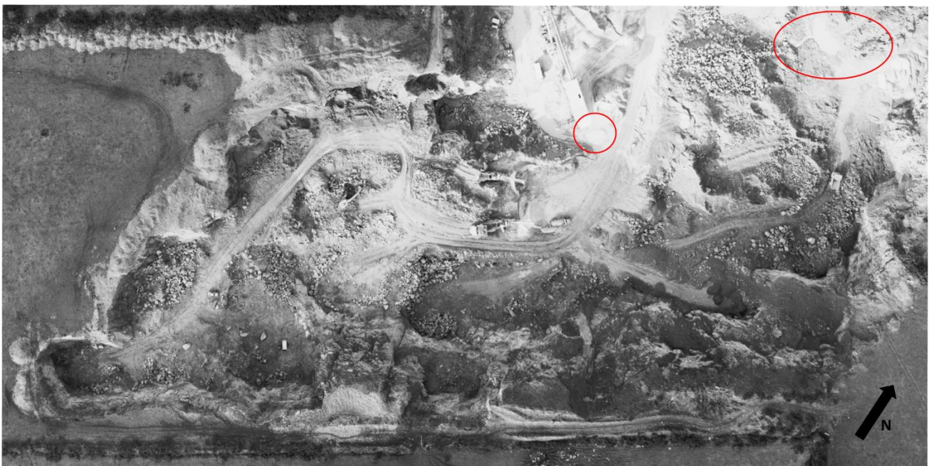
Figure 6.8: Area of Extraction Activities in 1991 (southern extent of Site, quarry floor is ca. 158-160 mAOD). Circled areas indicate potential locations of ponded water. Source of aerial imagery: Ordnance Survey Ireland.
