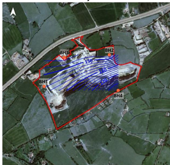
Figure 6.14: Groundwater Contours 2020 (aerial imagery from 2020). Groundwater elevations given in mAOD.
