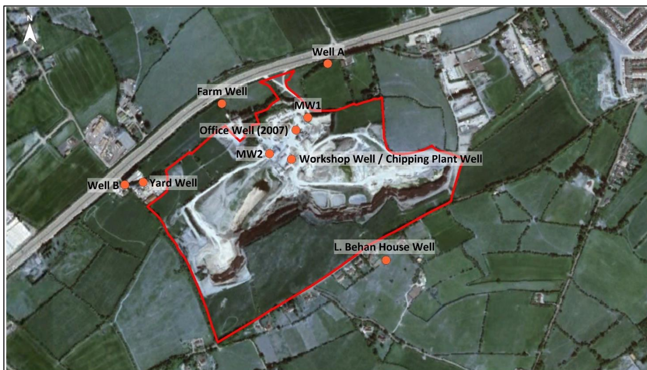
Figure 6.11: Location of Groundwater Wells Within and Immediately Adjacent to the Site 2006 to 2018 (Source of Aerial Imagery: Google Earth. Year: 2020).
